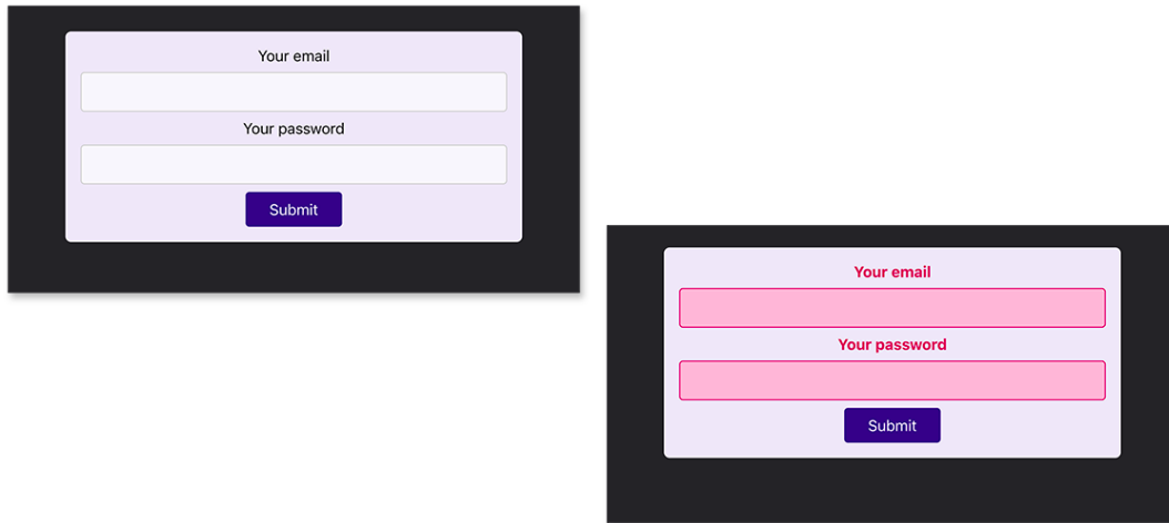
Figure 6.9: The final user interface with invalid input values highlighted in red
