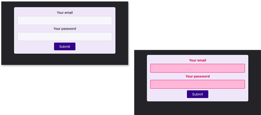
Figure 6.7: The final user interface with invalid input values highlighted in red
